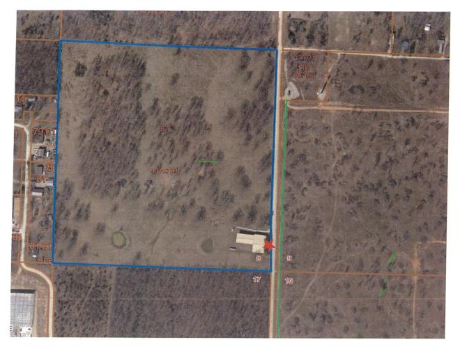
The red star is the approximate location of the desired water meter via the rural service agreement. The green line is the approximate location of the existing water line near the property on the east side of CR 2010.
