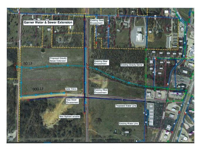
Note: Gravity sewer and manholes encompassed in red rectangles are shown for the purposes of future expansion and are not included in the scope of this revised project.
